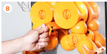
8 Remove the blade by pressing on the centre and pulling the handle towards you. Caution! Put the protector on the cutting zone.
