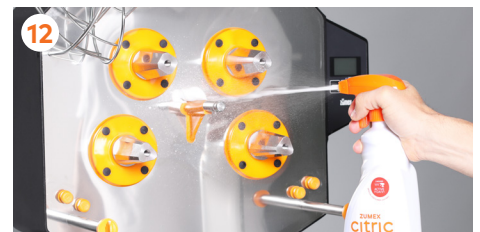
12 Clean the front zone of the machine, following the steps shown and removing all the particles which have adhered.
