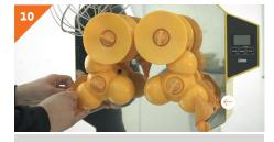
Pull off the peel ejectors.
