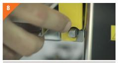
Press the lateral button to extract the steel bin. Removable in just one click.
