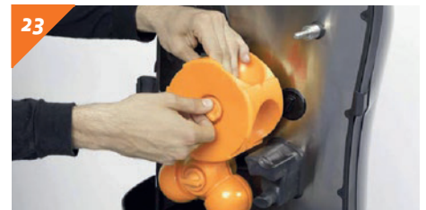
23 Tighten the securing knobs of the squeezing units.
