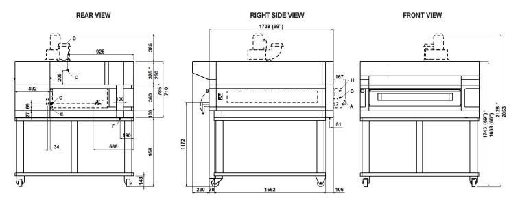
NOTE: The dimensions indicated in the views are in millimeters. \*Dimensions refer to the oversized hood.
