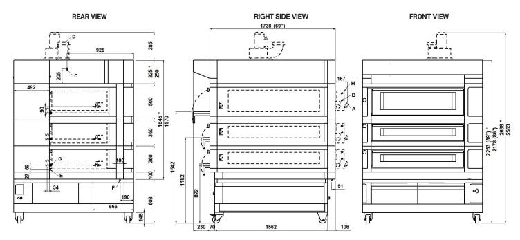
NOTE: The dimensions indicated in the views are in millimeters. \*Dimensions refer to the oversized hood.
